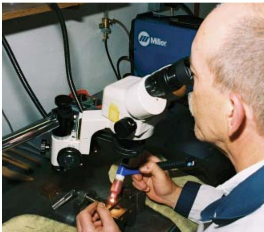
Joe Canfield, president of Five Star Tool Welding, microwelds a diecast insert for a lock mechanism. He dials power down to 1 A on his AC/DC gas-tungsten-arc/stick inverter to do this delicate work.
