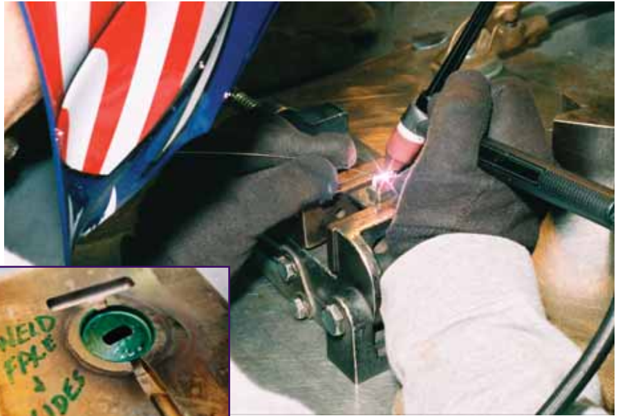
As he repairs a damaged injection mold insert, Five Star’s Joe Schultz uses his Syncrowave and \frac{1}{16} in. tungsten to precisely direct heat to the part. A common marker is used to indicate which parts of the tool need repair, such as cracks, worn edges and faces.
